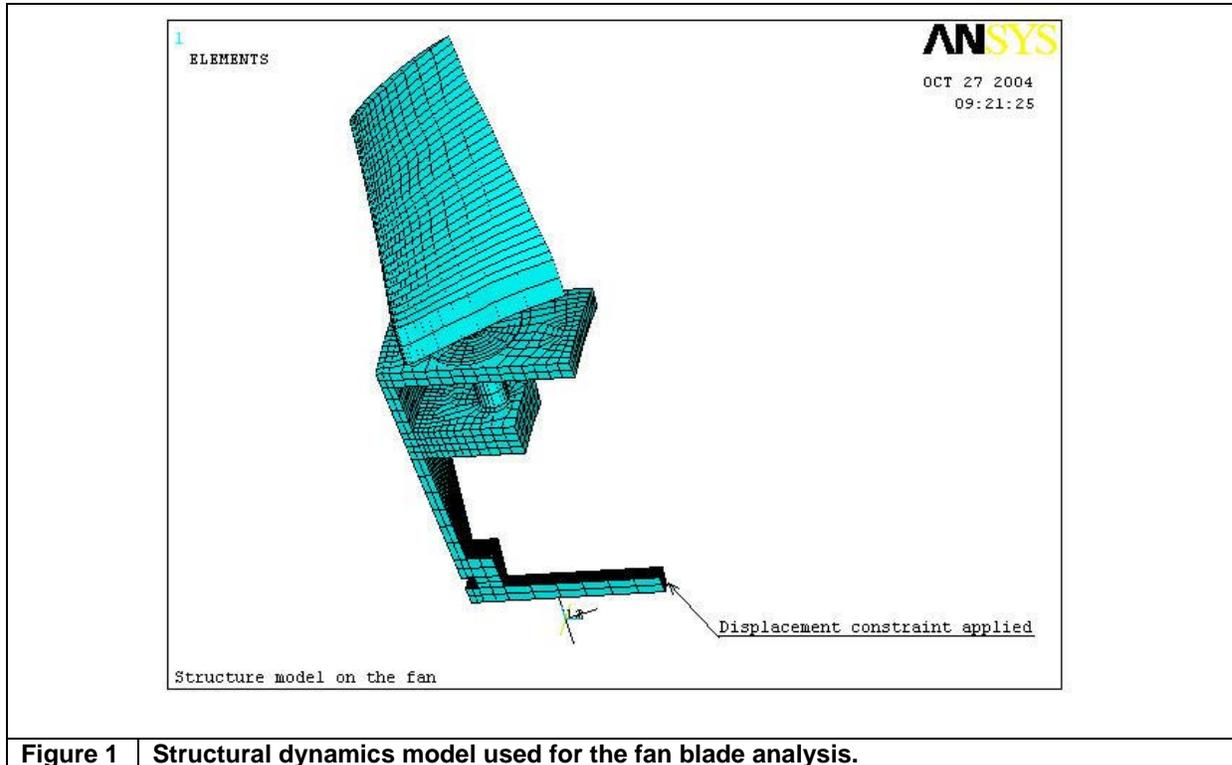
**Figure 1 | Structural dynamics model used for the fan blade analysis.**
