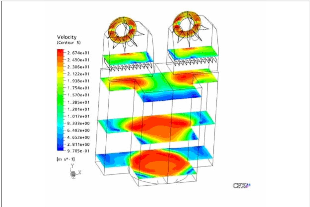
Figure 3a CFX-generated velocity contours
