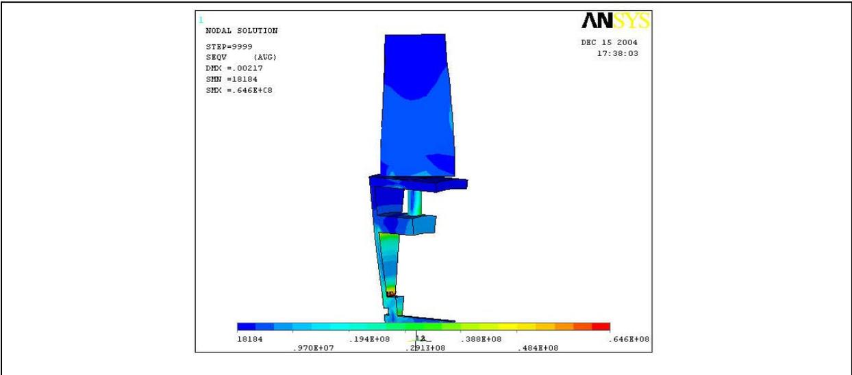
**Figure 13** | Real part of stress field (dirt build-up)
