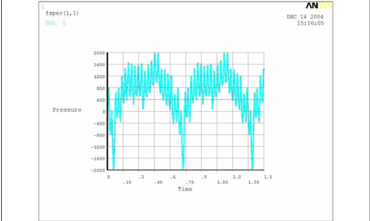
Figure 3b CFX calculated pressure oscillations at the fan blade at 890 rpm.
