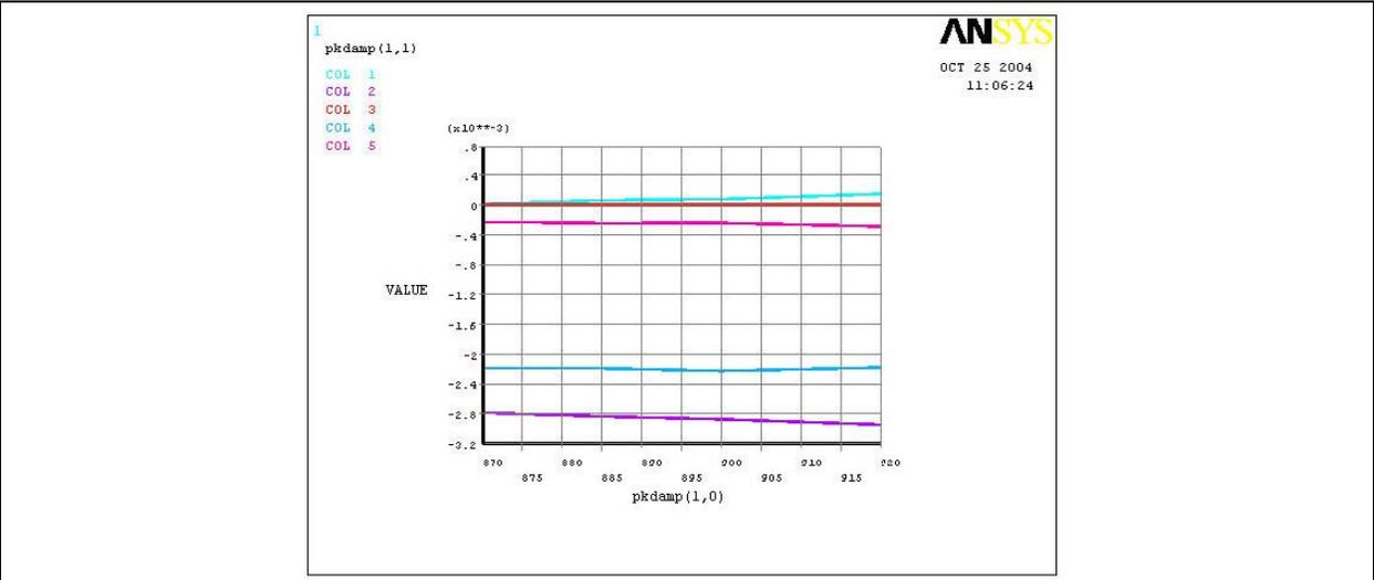
**Figure 8** | **Damping requirements for neutral stability for the 5 first modes in table 1.**
