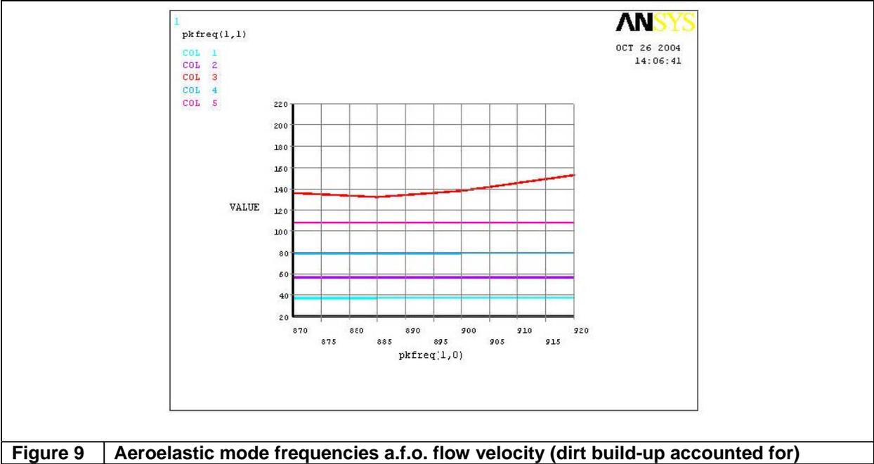
**Figure 9 Aeroelastic mode frequencies a.f.o. flow velocity (dirt build-up accounted for)**
