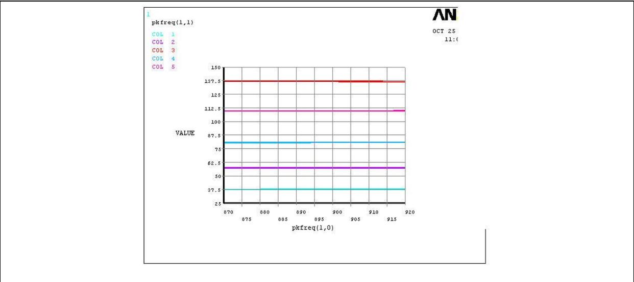
**Figure 7** | **Aeroelastic mode frequencies a.f.o. flow velocity.**
