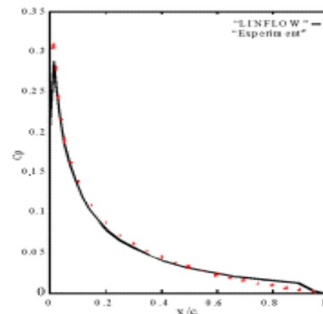
**Figure 3. Comparison of analysis and experimental results of dynamic pressure amplitude on the flutter boundary for a finite span wing.**
