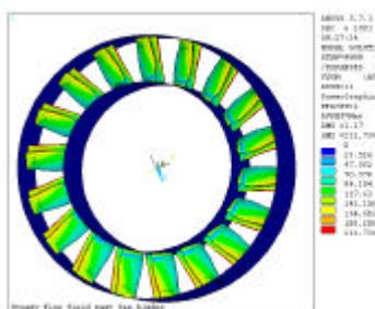
**Figure 2. Aeroelastic Analysis of double bladed fan (image courtesy of Fläkt Woods AB).**
